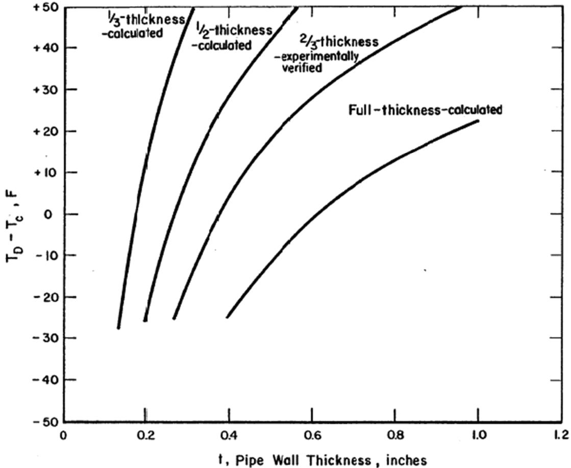
Figure 6. Transition temperature difference between DWTT ( $T_D$ ) and CVN ( $T_C$ ) at various pipe wall thickness and CVN coupon sizes [2]
