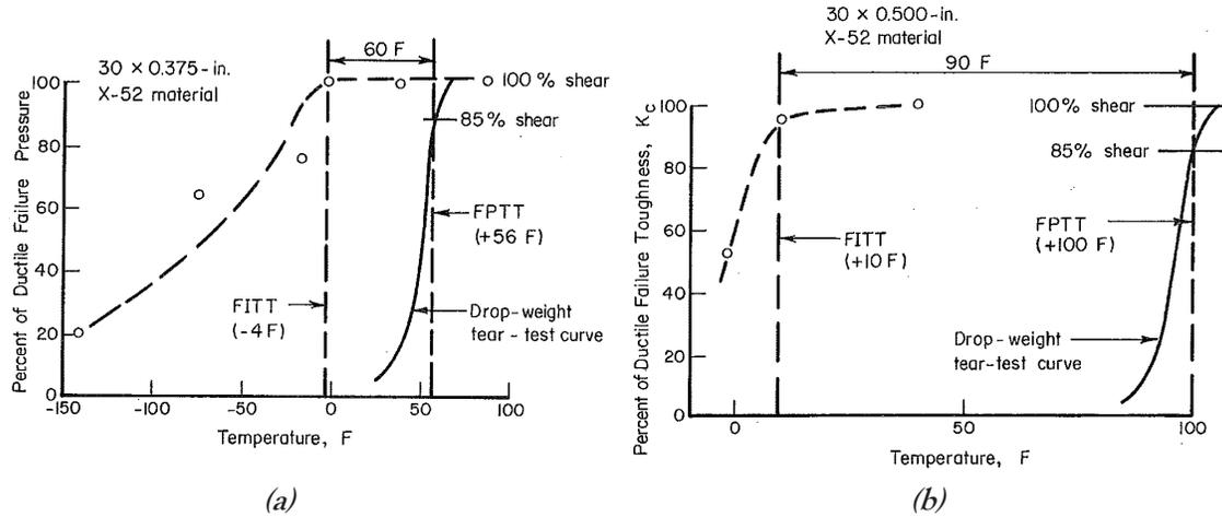
Figure 1. FITT and FPTT of through-wall flaws from Battelle's tests [3]
