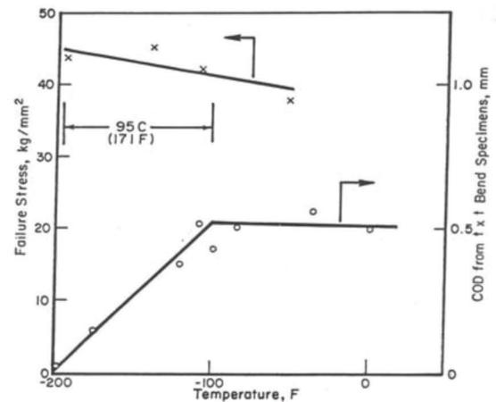
Figure 5. CTOD tests and full-scale burst test with surface crack [6]
