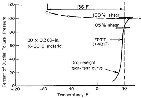
Figure 2 FITT and FPTT of surface flaws from Battelle's tests [3]
