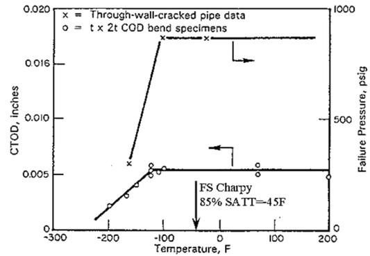
Figure 3. FITT of Through-wall crack and CTOD Tests [4]
