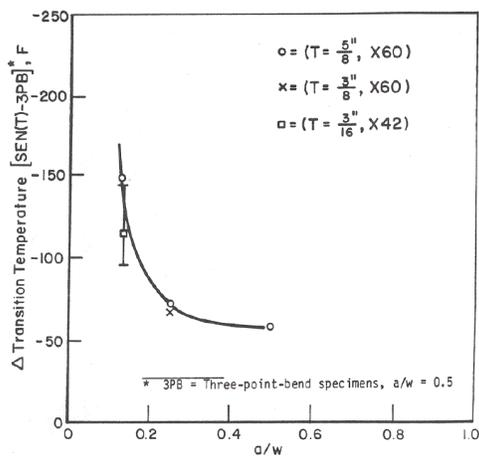
Figure 4. Comparison of FITT-S and FITT-H through SEN(T) and SEN(B) [5]
