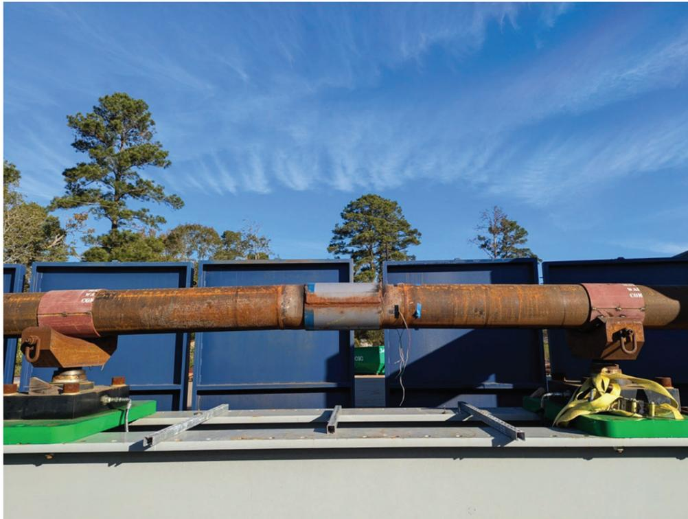
Figure 9. Sample 1 (Type A Compression Sleeve) post test.
