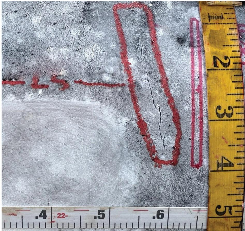
Figure 3. Photograph of the Sample 3 indication selected for repair using composite.
