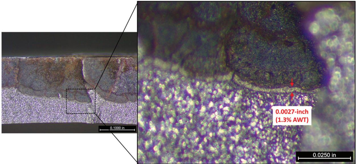
Figure 18. Photograph at the base of the Sample 3 indication (Composite Repair) showing area of growth. Original magnification: Left: 12.8x, Right: 48x.
