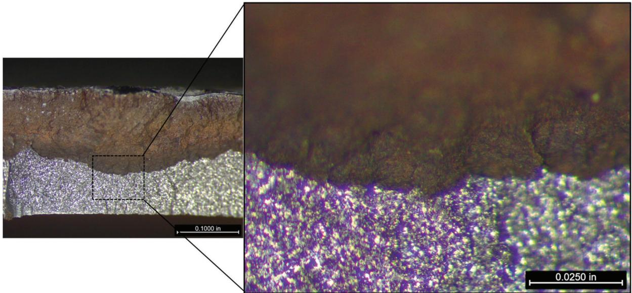
Figure 16. Photograph at the base of the Sample 2 indication (Type A Compression Sleeve Repair) showing no growth. Original magnification: Left: 12.8x, Right: 48x.
