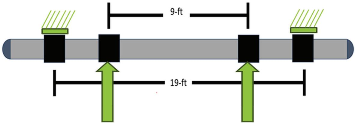
Figure 5. Four-point bending sample setup
