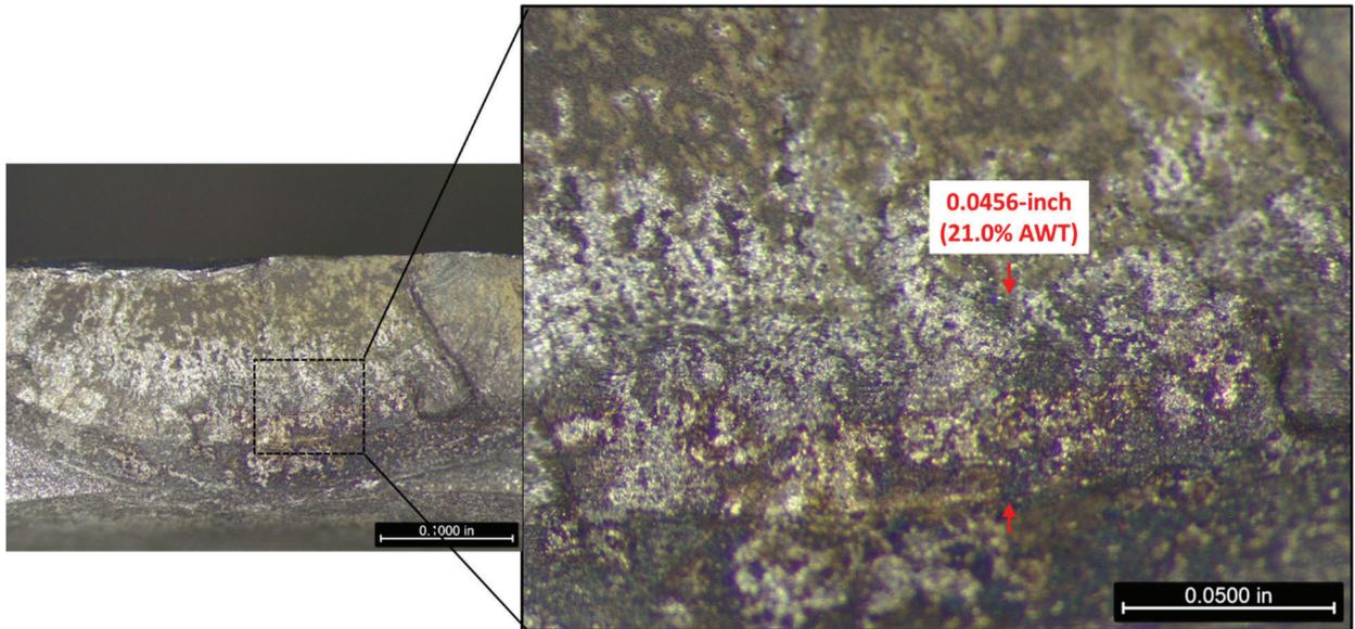
**Figure 22.** Photograph at the base of the Sample 4 indication (Unreinforced) showing area of growth. Original magnification: Left: 12.8x, Right: 25.6x.
