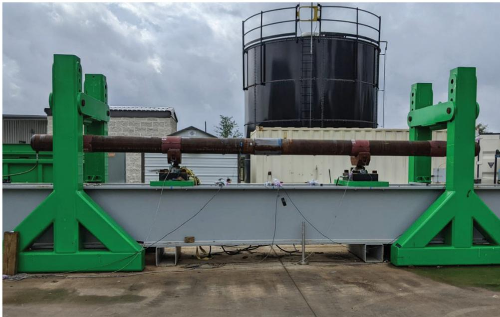
Figure 6. Sample 1 (Type A Compression Sleeve) in test setup.
