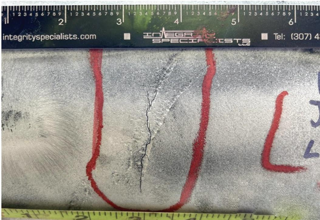
Figure 1. Photograph of the Sample 1 indication selected for repair using a Type A Compression Sleeve.
