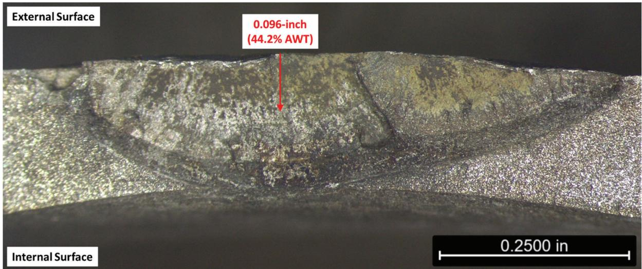
Figure 20. Photograph of the Sample 4 indication after breaking open and cleaning (Unreinforced). Original magnification is 6x.
