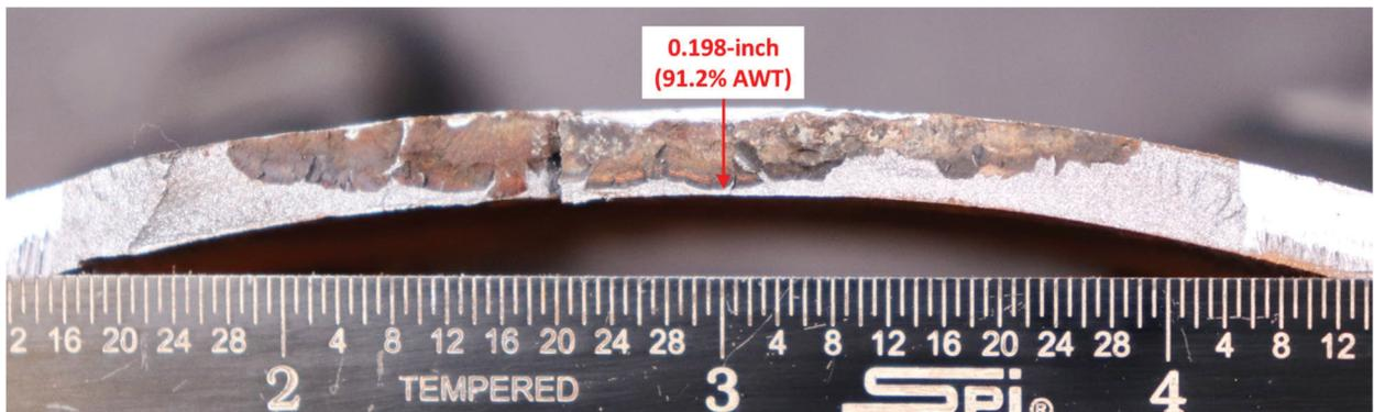
Figure 13. Photograph of the Sample 1 indication after breaking open (Type A Compression Sleeve Repair). Major numbered scale divisions are inches.
