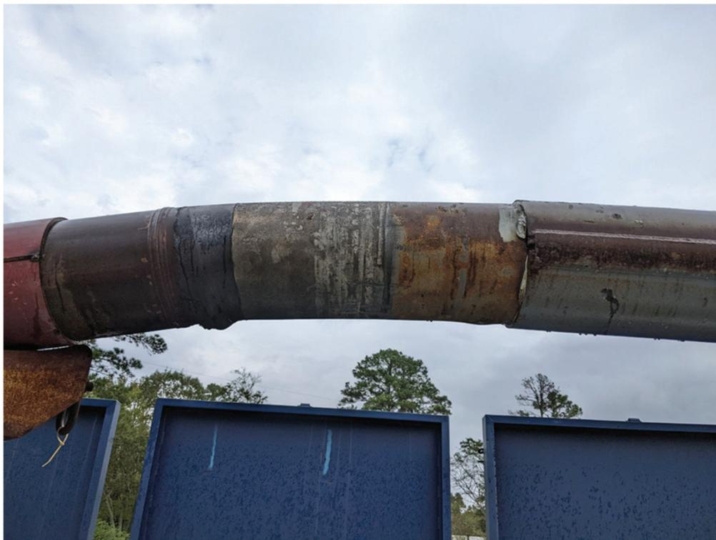
Figure 10. Sample 2 (Type A Compression Sleeve) post test.
