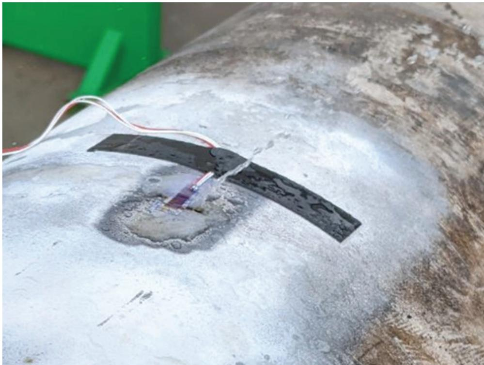
Figure 8. Sample 4 (Unreinforced) leak location.
