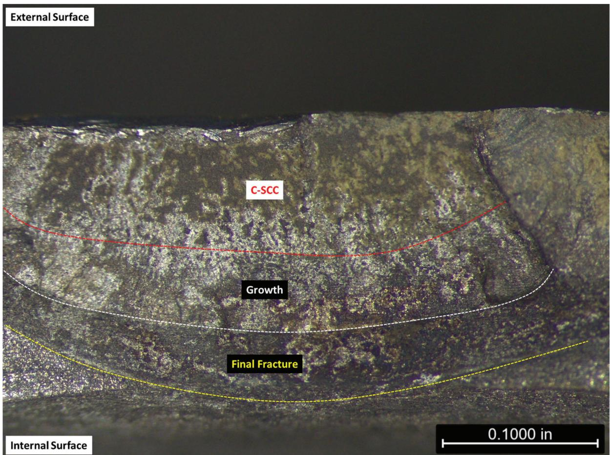
Figure 21. Photograph of boundaries present on the Sample 4 indication after breaking open and cleaning (Unreinforced). Original magnification is 12.8x.
