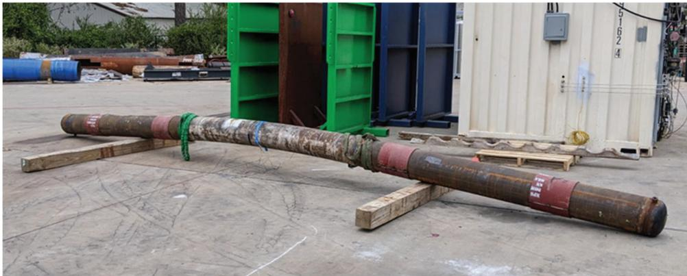
Figure 12. Sample 4 (Unreinforced) plastic deformation post test.
