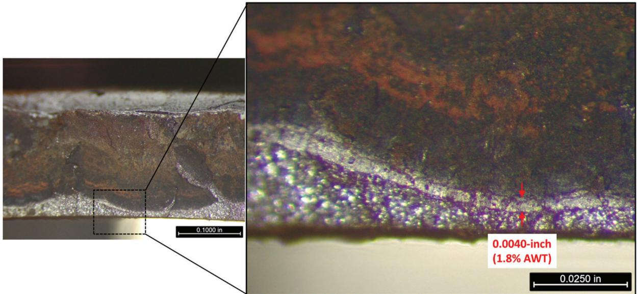
Figure 14. Photograph at the base of the Sample 1 indication (Type A Compression Sleeve Repair) showing area of growth. Original magnification: Left: 12.8x, Right: 48x.
