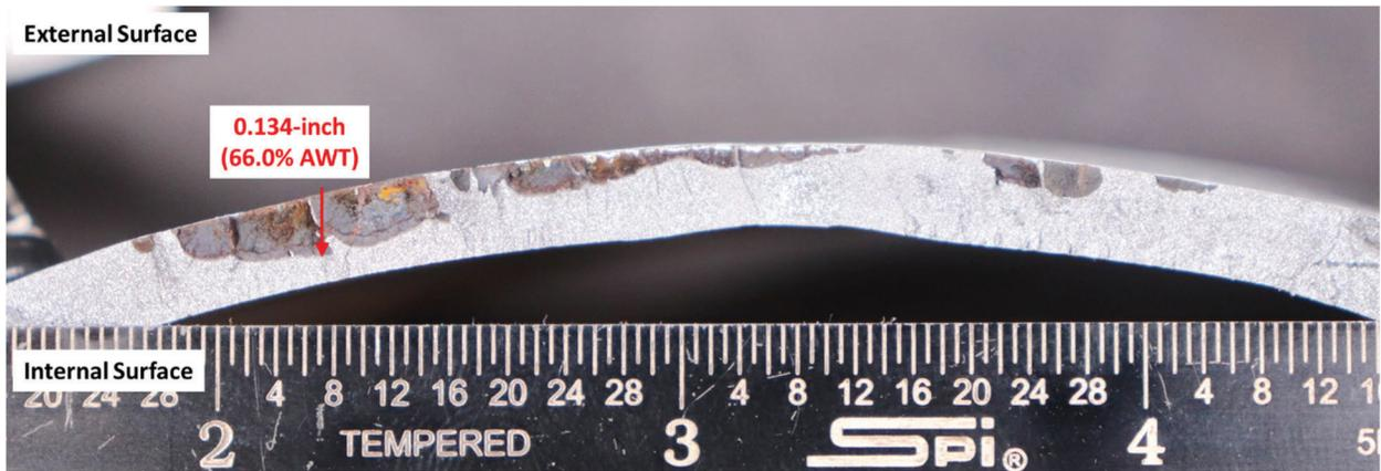
Figure 17. Photograph of the Sample 3 indication after breaking open (Composite Repair). Major numbered scale divisions are inches.
