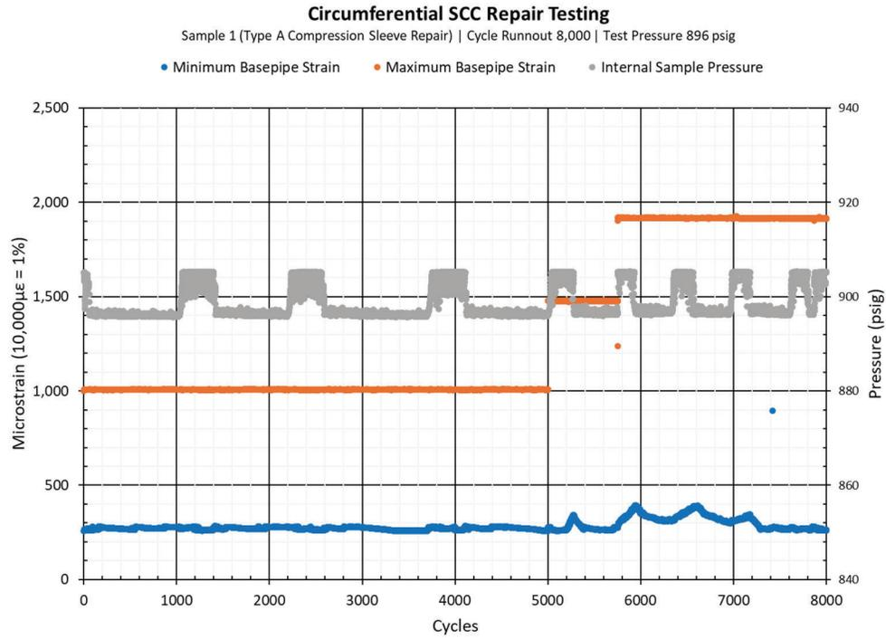
Figure 7. Sample 1 (Type A Compression Sleeve) cycle strains and internal pressure during bend cycling.
