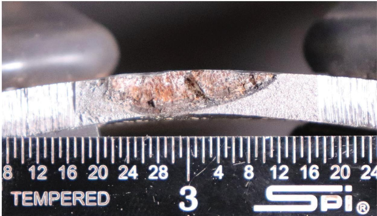
Figure 19. Photograph of the Sample 4 indication after breaking open (Unreinforced). Major numbered scale divisions are inches.
