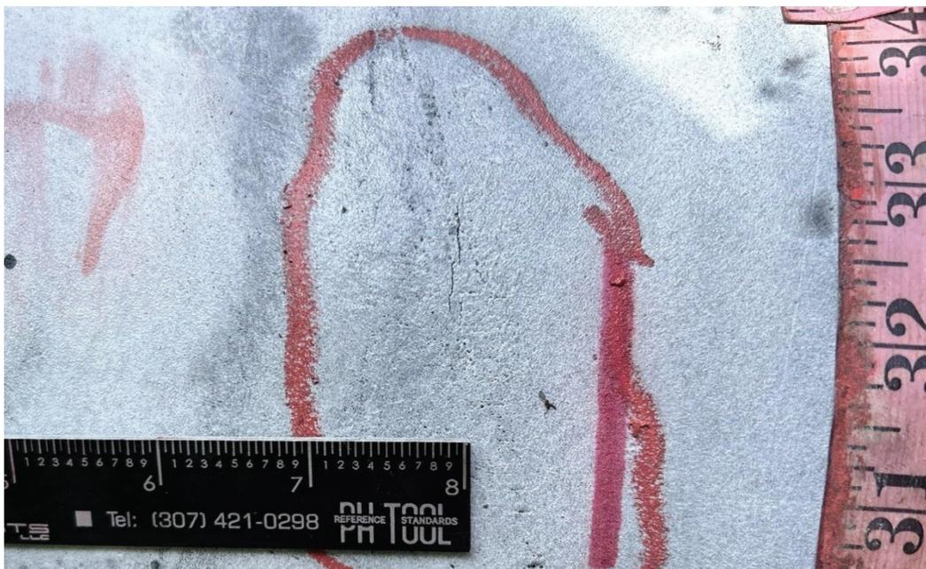
Figure 4. Photograph of the Sample 4 indication selected for unreinforced sample.
