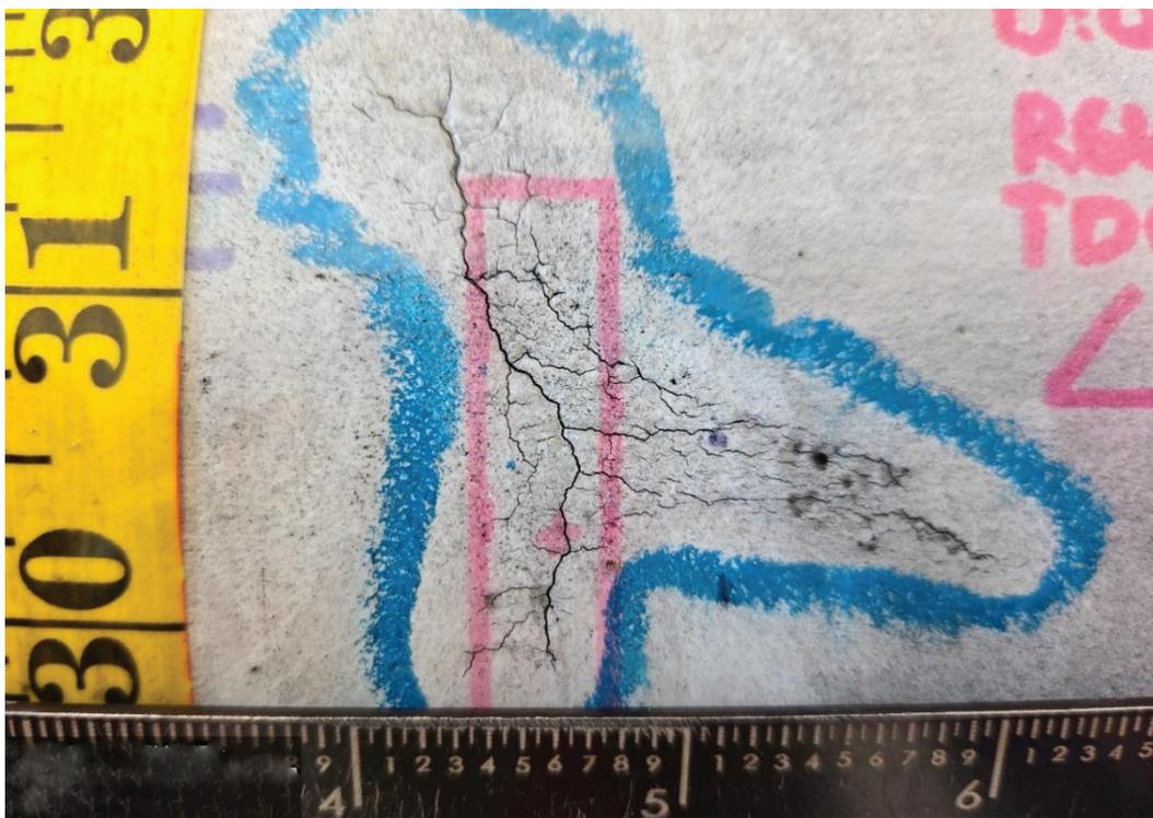
Figure 2. Photograph of the Sample 2 indication selected for repair using a Type A Compression Sleeve.
