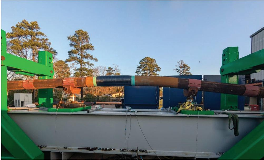
Figure 11. Sample 3 (Composite Repair) post test.
