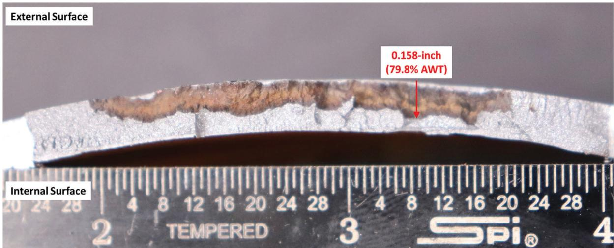
Figure 15. Photograph of the Sample 2 indication after breaking open (Type A Compression Sleeve Repair). Major numbered scale divisions are inches.
