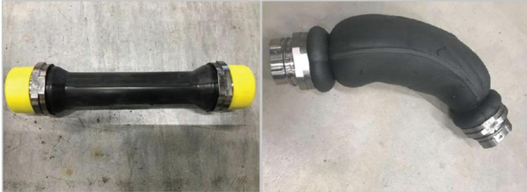
**Figure 5:** Cable before (L) and after (R) CO<sub>2</sub> exposure testing
