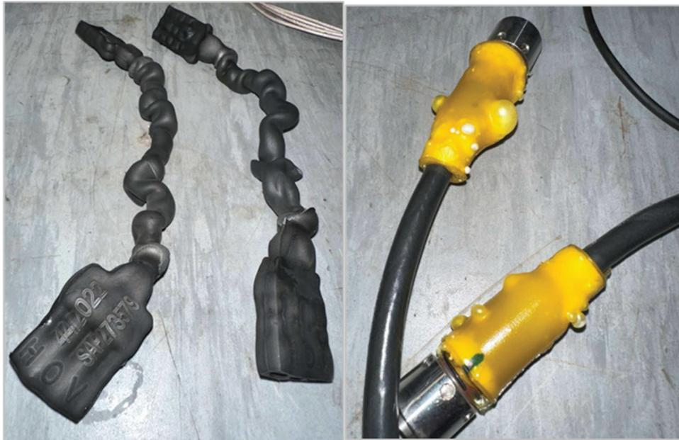
Figure 7: Cables after CO<sub>2</sub> exposure testing
