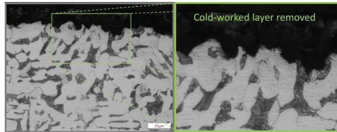
**Figure 5:** Example of superficial cold-worked layer removed
