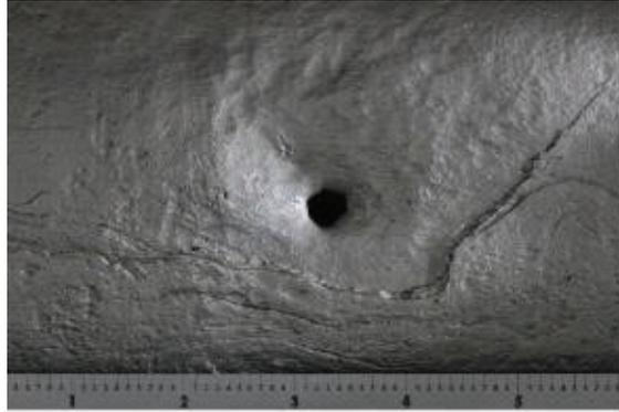
**Figure 3:** Corrosion feature that leaked
