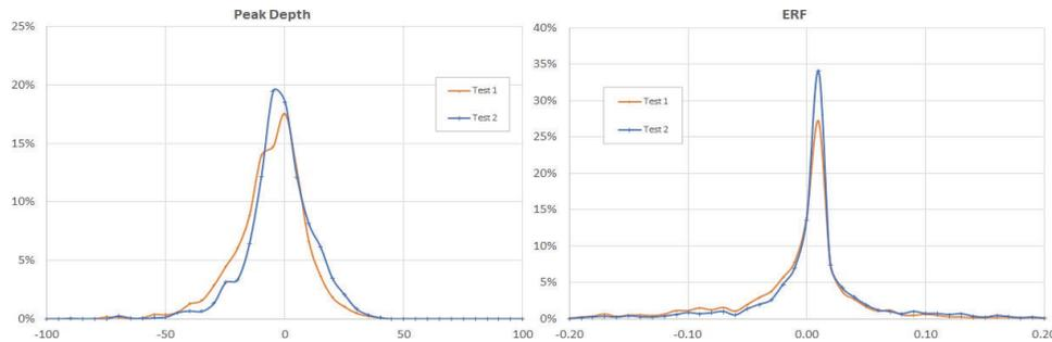
Figure 10: Relative frequency distributions for  $d_{max}$  and ERF differences in T1 and T2 - ILI TP3
