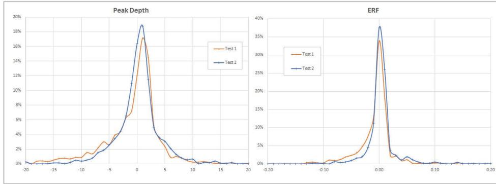
Figure 8: Relative frequency distributions for  $d_{max}$  and ERF differences in T1 and T2 - ILI TP 1
