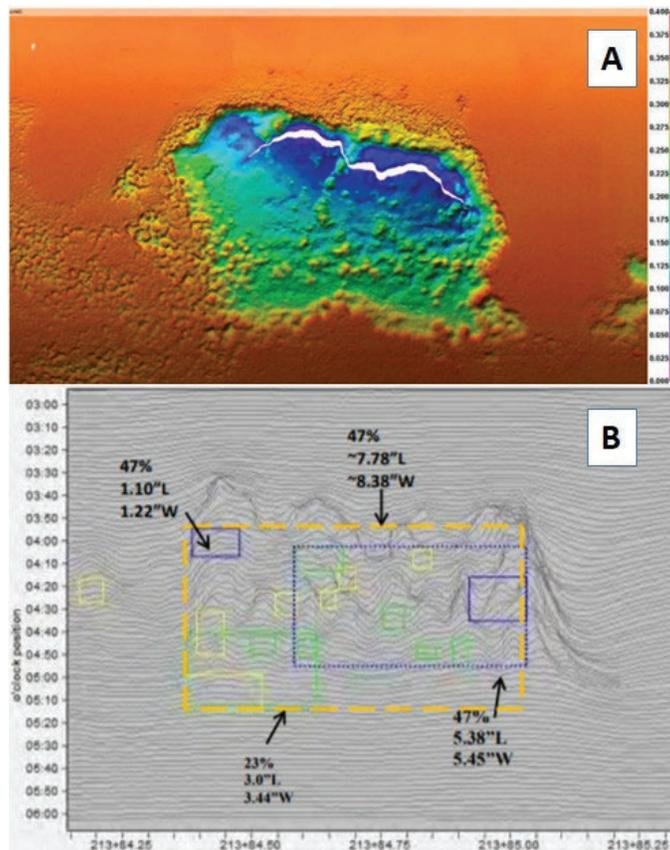
Figure 2: (a) Ruptured corrosion feature (b) MFL signal data of the same feature before the failure occurred
