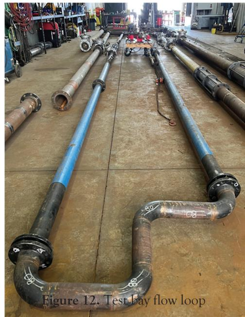
Figure 12. Test bay flow loop
