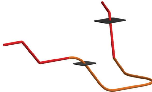
Figure 18. Pipeline layout, orange indicating the portion inspected via the tether application in 2017 (not to scale)
