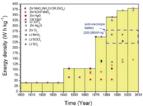
Figure 5. Battery energy density timeline energy densities remain quite similar, configurations are being utilized.
