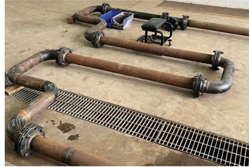
Figure 13. Final flow loop test setup
