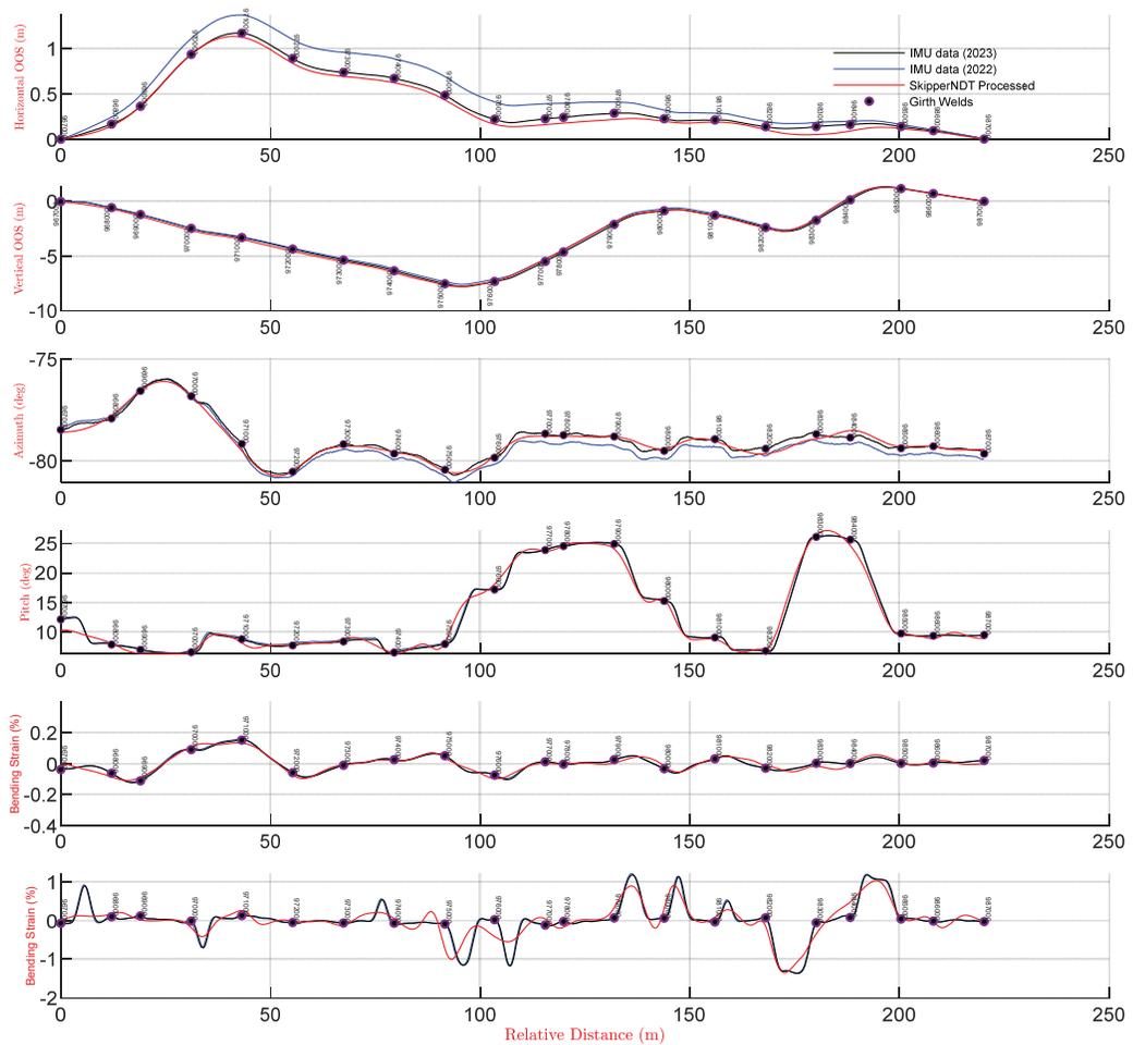
**Figure 5:** Top to bottom: a) Horizontal out-of-straightness profile, b) Vertical out-of-straightness profile, c) Azimuth profile, d) Pitch profile, e) Horizontal bending strain profile and f) Vertical bending strain profile at Site 1.
