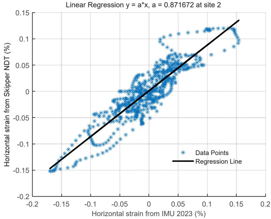
**Figure 10:** Linear regression between magnetic-based horizontal strain and IMU horizontal strain at Site 2.
