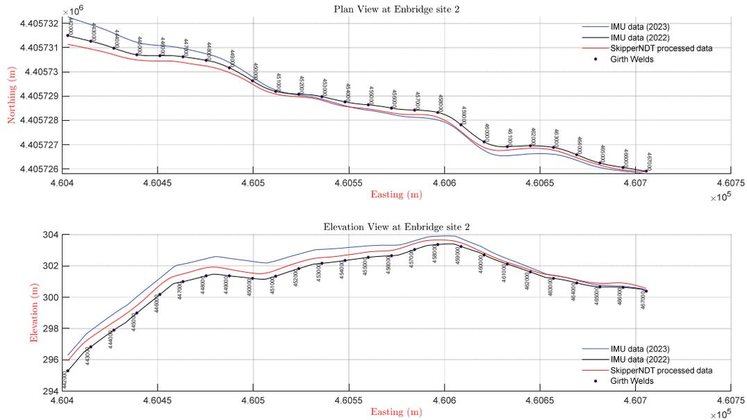
Figure 6: Plan and elevation views at Site 2.
