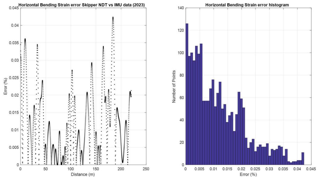
**Figure 9:** Horizontal bending strain error between magnetic-based and IMU 2023 at Site 1. Median = 0.00979%, STD = 0.00958%
