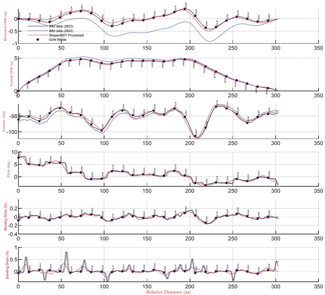
**Figure 7:** Top to bottom : a) Horizontal out-of-straightness profile, b) Vertical out-of-straightness profile, c) Azimuth profile, d) Pitch profile, e) Horizontal bending strain profile and f) Vertical bending strain profile at Site 2
