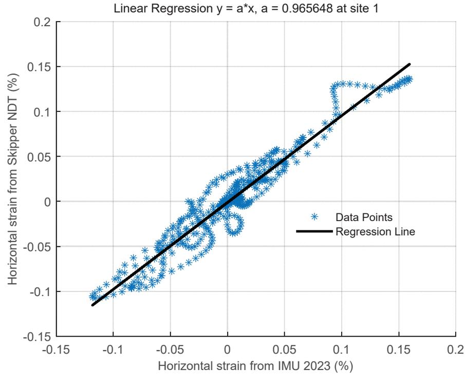
**Figure 8:** Linear regression between magnetic-based horizontal strain and IMU horizontal strain at Site 1.
