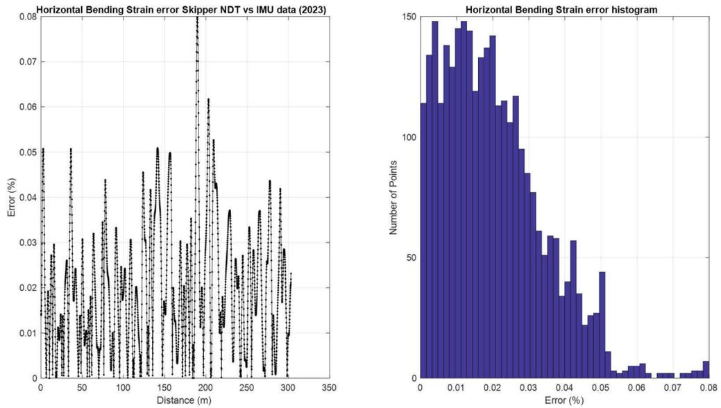
**Figure 11:** Horizontal bending strain error between magnetic-based and IMU 2023 at Site 2. Median = 0.0171%, STD = 0.0131%.
