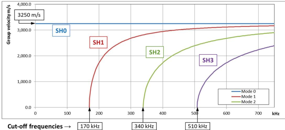
Figure 3. Dispersion curves for a mild steel 9.6mm thick plate
