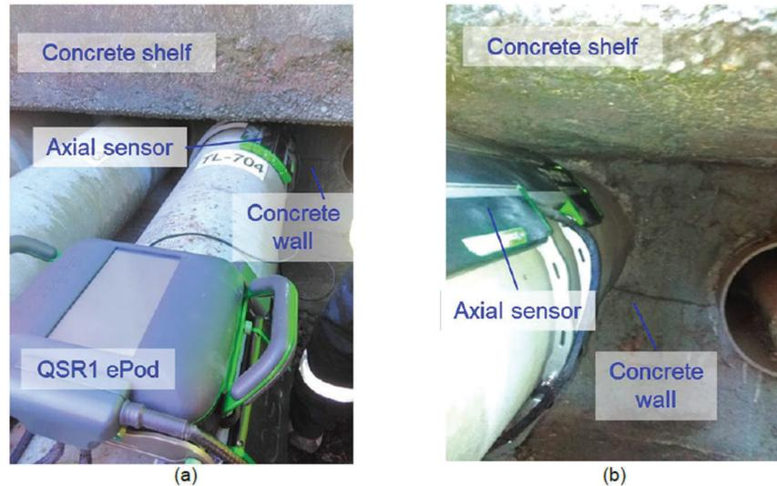
Figure 13. Scanning configuration at concrete wall penetration. (a) the QSR1 electronics pod controls the Axial sensor and traction unit (not visible). (b) the Axial sensor clearance beneath shelf extension and proximity to concrete wall.
