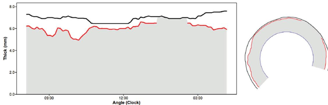
Figure 15. Axial scan results from Test Position 1 under concrete shelf
