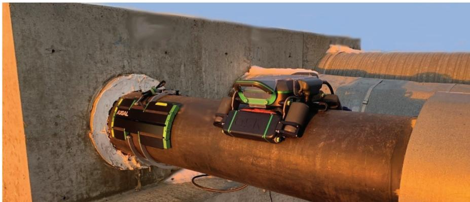
Figure 4. QSR1 and QSR Axial scanning systems at concrete wall penetration
