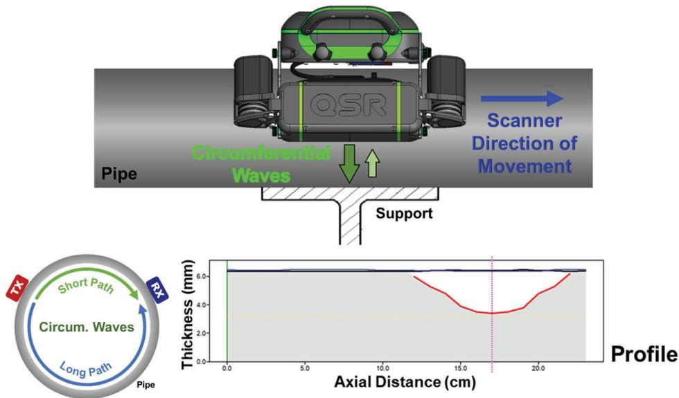
Figure 5. Circumferential scan movement and example profile result
