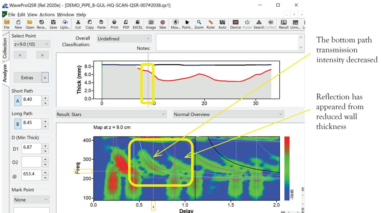
Figure 7. Manual analysis of transmission and reflection traces
