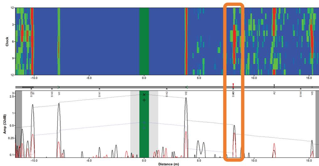
Figure 10. Guided wave screening results indicating significant wall loss
