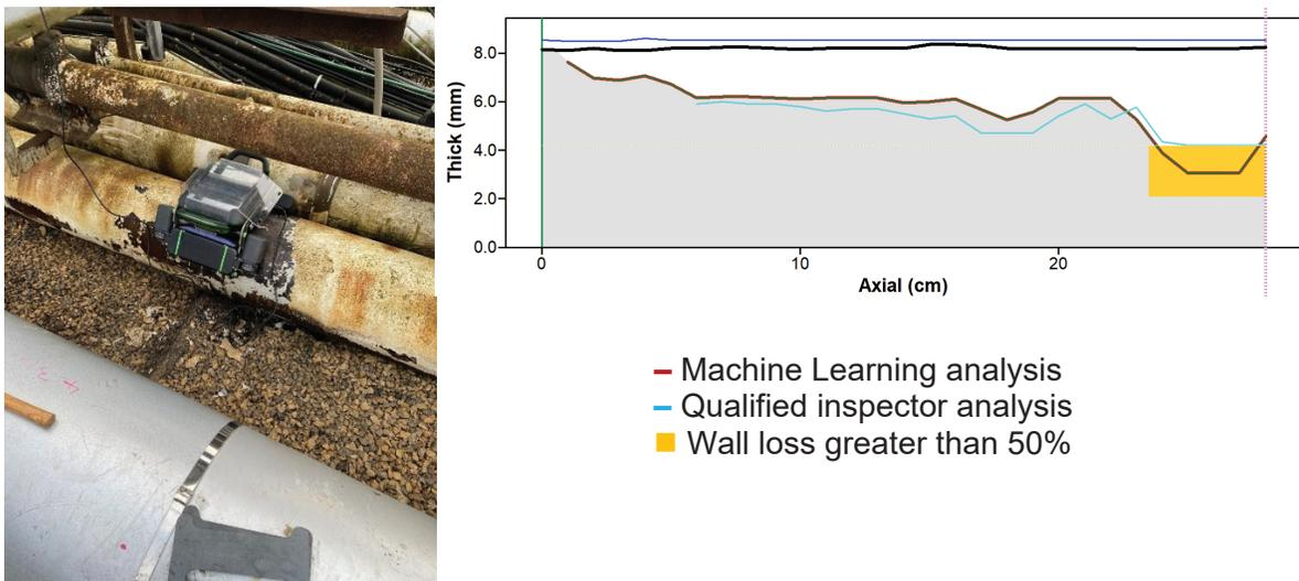
Figure 11. QSR1 scanning in-progress and profile results
