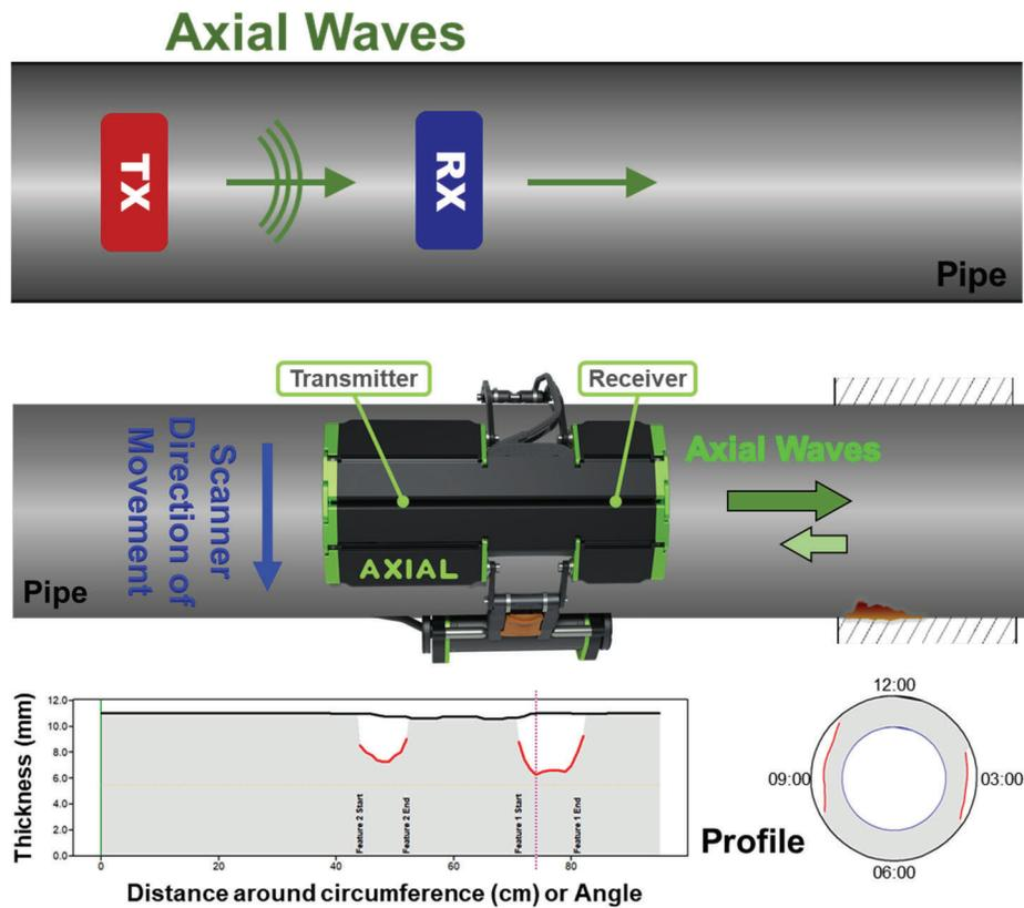
Figure 6. Axial scan movement and example profile result
