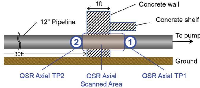
Figure 14. Side view sketch layout of 12" pipe QSR test positions
