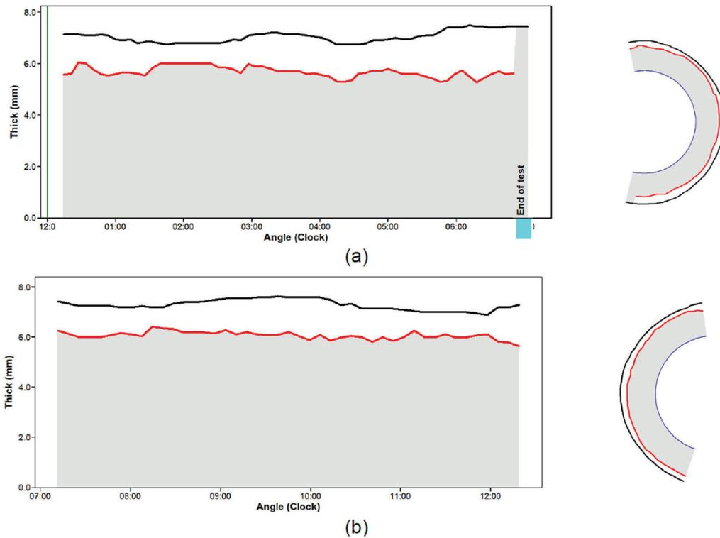
Figure 17. Axial scan results from Test Position 2
