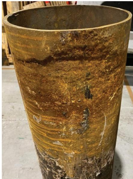
Figure 12. 12" pipe removed from service with significant external wall loss
