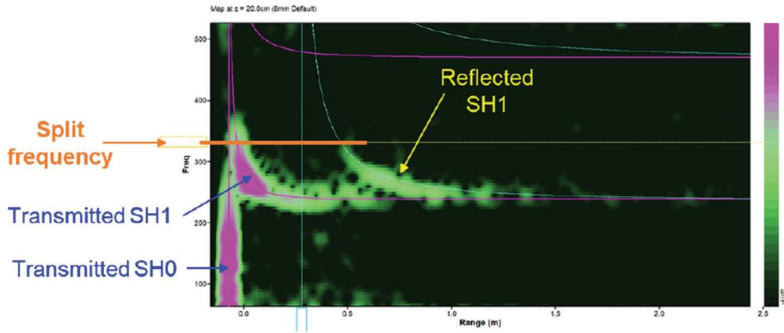
Figure 16. Axial split frequency analysis from Test Position 1
