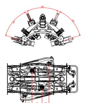
Unlike existing technologies, the ART vPush only needs access to the top half of the pipe, greatly reducing or eliminating the need for dredging.
