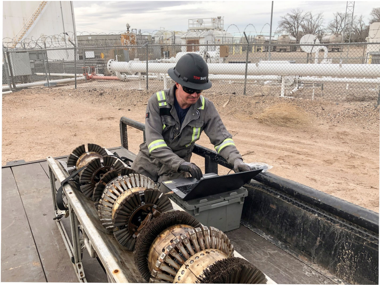
FIGURE 4: ILI FIELD TECH. WITH THE MULTIPLE DATASET (MDS) TOOL
