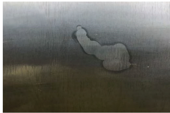
Figure 13: Nital Etching for Figure 10 Spool
