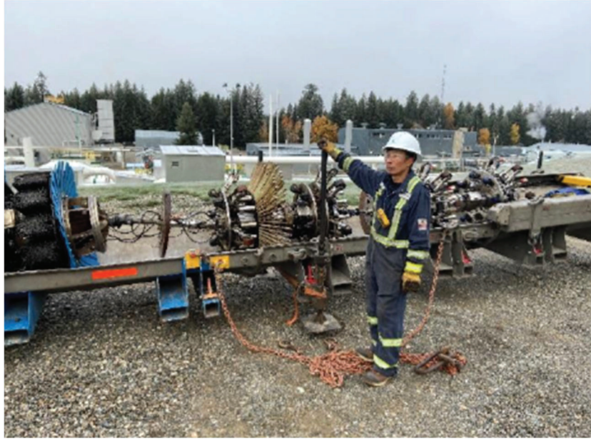
Figure 9: 36" AXISS EPS preparing to launch for first field trial
