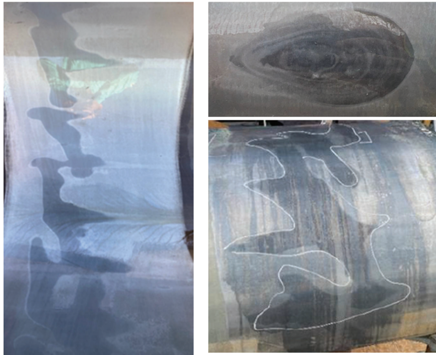
Figure 2: Hardness anomalies verified in ditch <327 BHN
