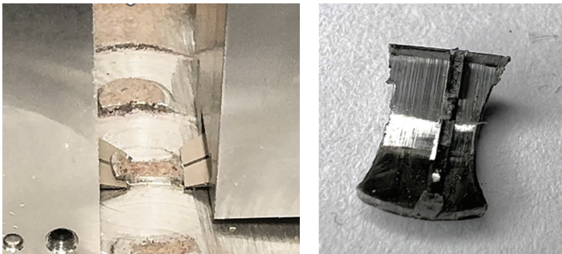
Figure 2. Left: a Zoom-in of the BTM blade cutting into a test island. Right: chip formed after a BTM test.
