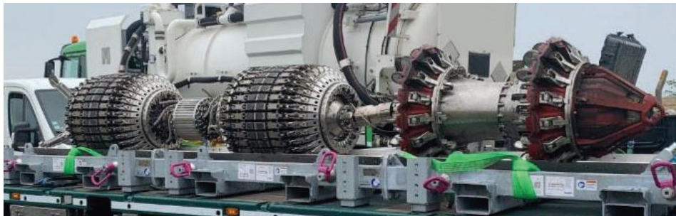
Figure 3. Picture of an EMAT-C Ultra tool at job site before launching
