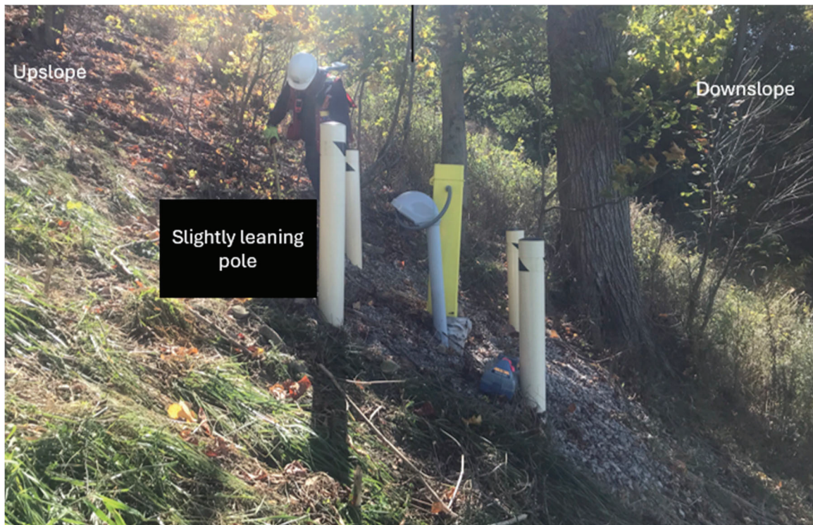
Figure 8. View of SAA casing at case study site that was installed during drainage mitigation.
