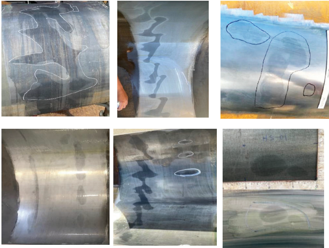
Figure 1. Example of different hardness anomaly morphologies observed on the pipe surface
