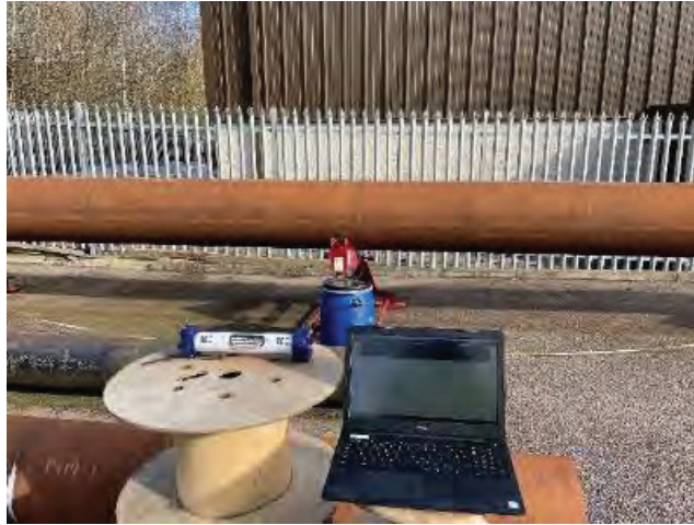
Figure 6. EMRx positioned 1m from pipe center
