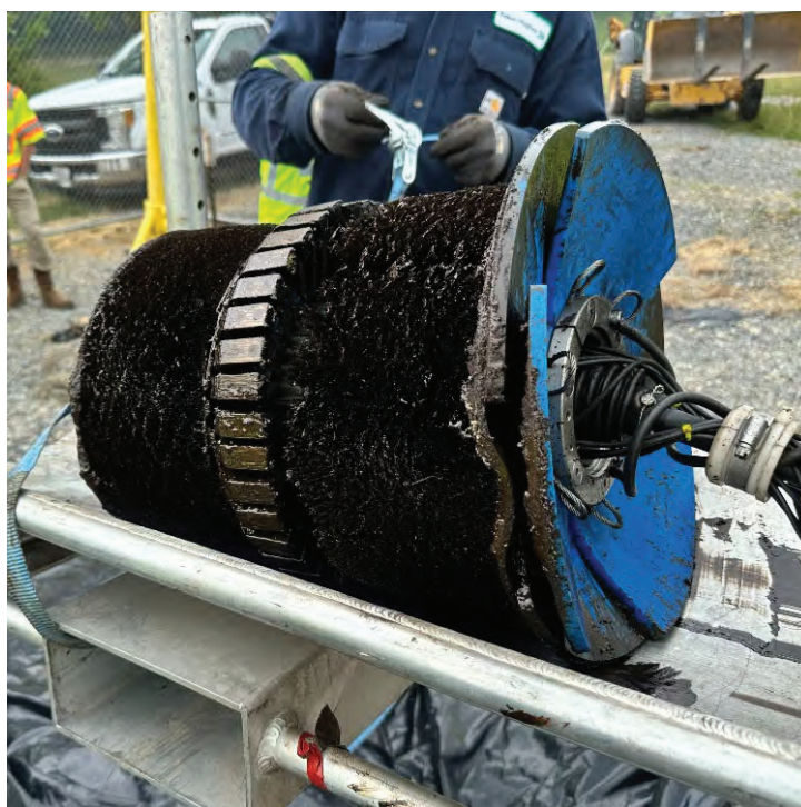
Figure 6. Debris in ILI tool after survey, a potential source of NORMs
