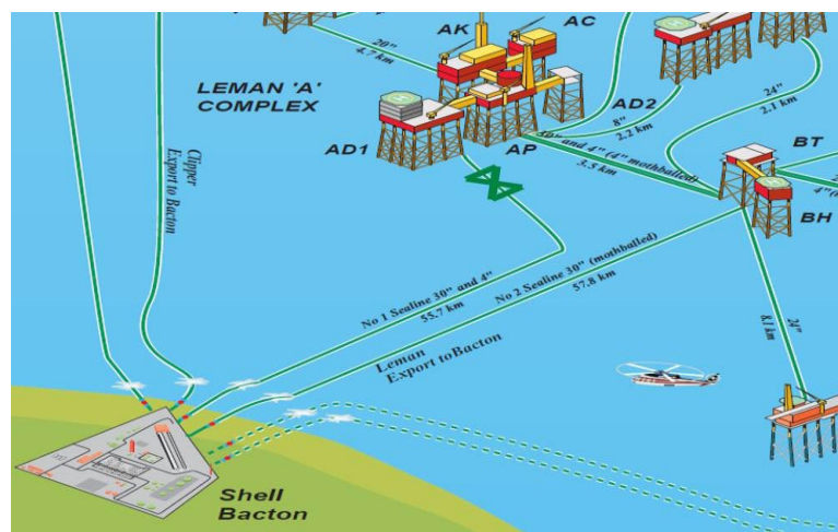
Figure 1: Leman – Bacton pipeline system overview
