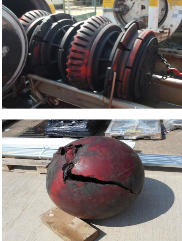
Figure 6: Recovered damaged sphere and rescue pig
