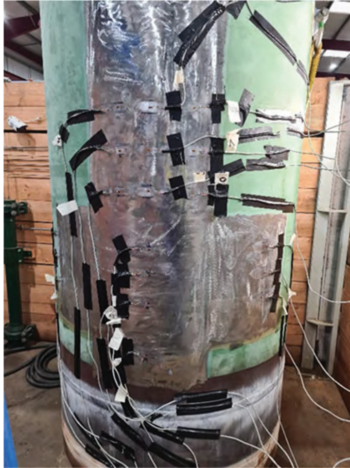
Figure 4. Installation of strain gauges by DNV during FAT
