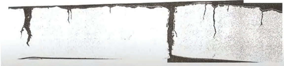
Figure 10. Micrograph of a metallographic cross-section taken through a failed section of pipe, Figure T-4 Reference [20].
