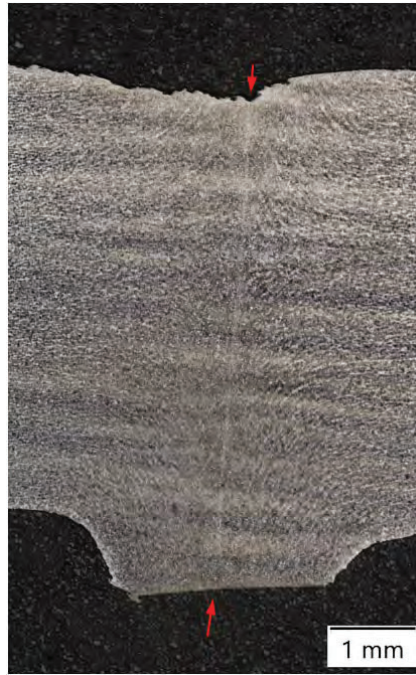
Figure 10. Representative image of the seam weld cross section at Site 134. The bondline is highlighted by the red arrows.
