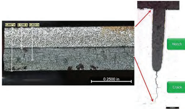
Figure 5. Microcracking observed at the base of an EDM notch (meridional and cross-section views)
