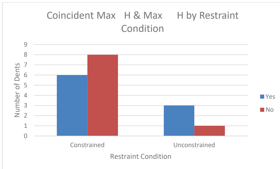
Figure 3. Summary of Coincident Maximum Circumferential Stress and Maximum Change in Circumferential Stress as a function of Restraint Condition
