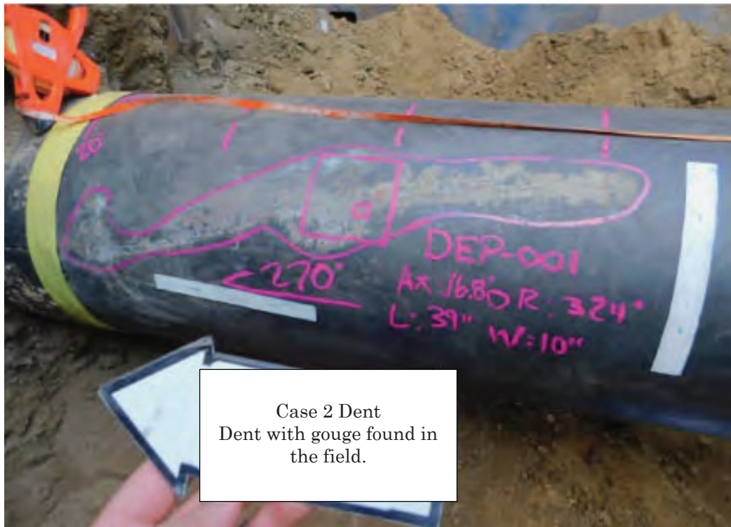
Figure 7. Case 2 Dent Field Findings
