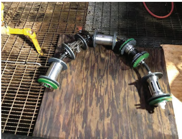
Figure 2 - Surveyor UT tool prior to launch
