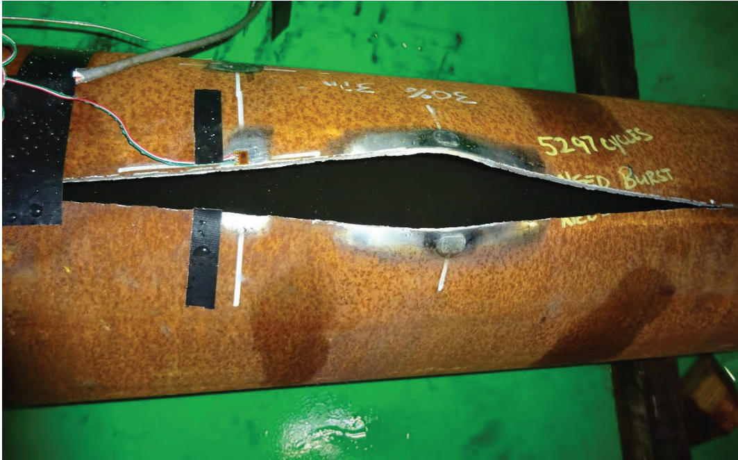
Figure 1. Photograph of a burst test to evaluate a crack-like feature
