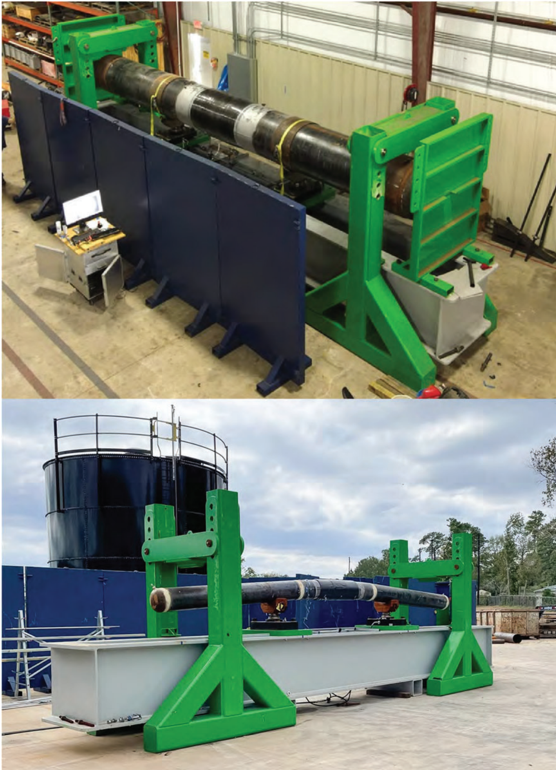
Figure 5. Four-point bend frame (3 million ft-lb (4.1 million N-m) capacity) (30-inch pipe shown in [top]; 12-inch pipe after bend test [bottom])
