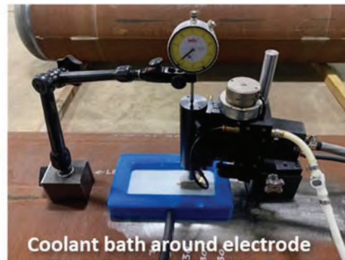
Figure 7. Photographs showing the installation of an EDM notch
