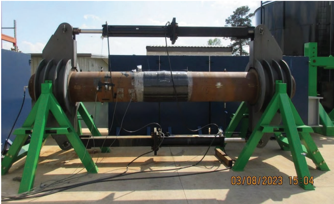
Figure 6. High strain bending frame (800,000 ft-lb (1.1 million N-m) capacity)
