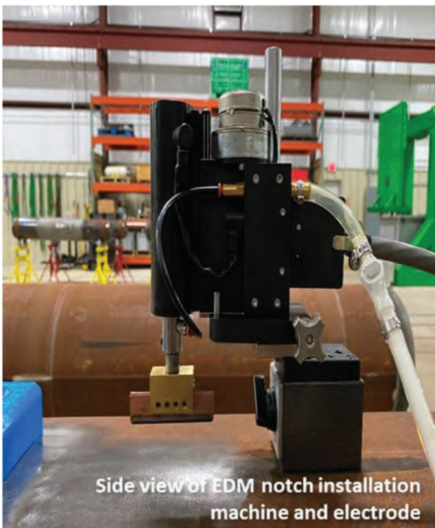
Figure 7. Photographs showing the installation of an EDM notch
