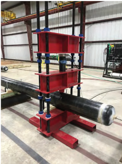
Figure 11. Photographs showing the dent installation test rig
