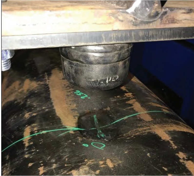
Figure 19. View of simulated dent after indenter removal
