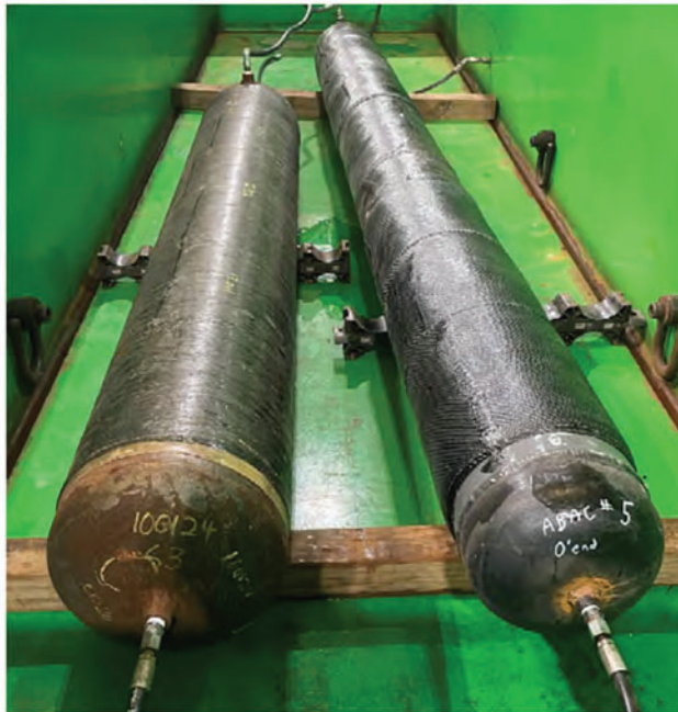
Figure 1. Pipe 6 before pressure cycling (left) and pinhole leak at air bubble in Pipe 3
