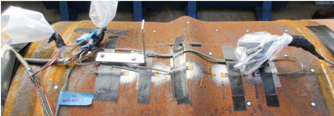
Figure 1. Unreinforced wrinkle with instrumentation
