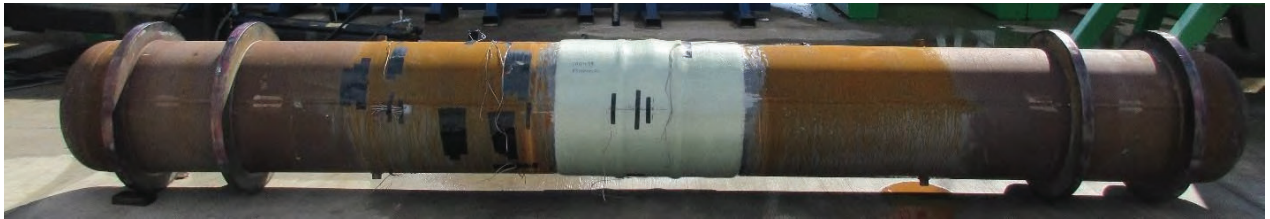
Figure 4. Wrinkle sample reinforced with E-glass composite wrap
