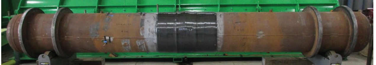
Figure 5. Wrinkle sample reinforced with carbon fiber composite wrap
