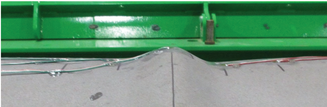
Figure 1. Unreinforced wrinkle with instrumentation
