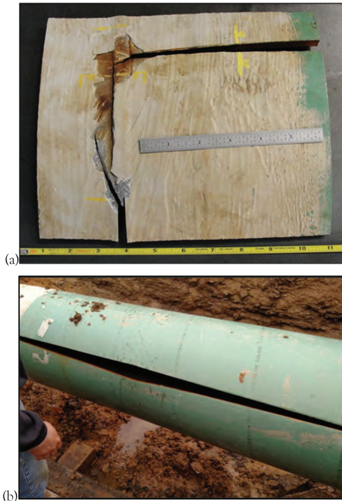
Figure 2(a-b). Case 2 – Investigative failure photo (a) Seam failure of 2015 installed pipe under hydrostatic test (b)
