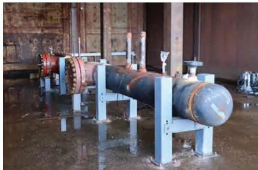
Figure 18. WP1 Tee Fatigue Test Vessel
