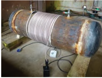
Figure 16. Heating of defect on hydrogen burst test vessel
