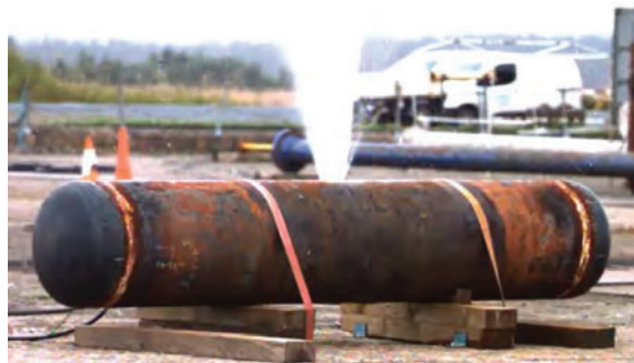
Figure 15. Hydrostatic Burst Test
