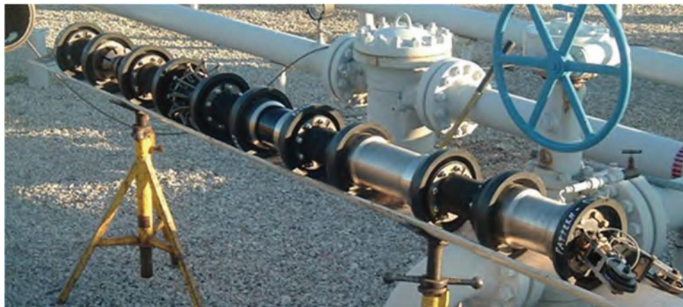
Figure 7. 8-inch MFL Ammonia ILI Tool (prior to launch)
