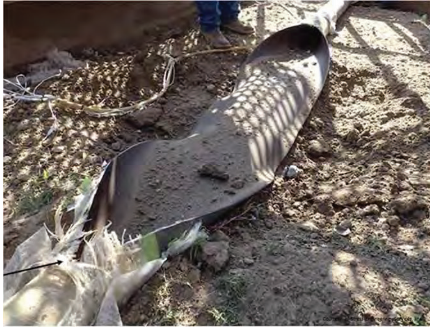
Figure 3. Photographs showing the post-test response of a “soft” arrest response.
