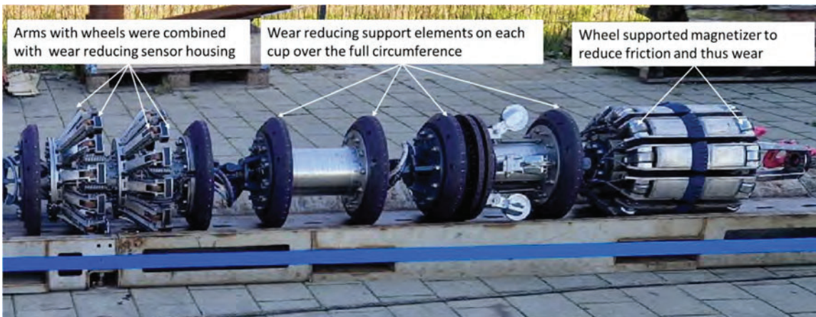
Figure 4. Wear reducing design optimizations on the different ILI tool segments.
