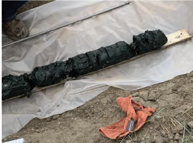
Figure 22. 4” tool after inspection of the 4” segment. Note the amount of paraffin attached to the tool sections.
