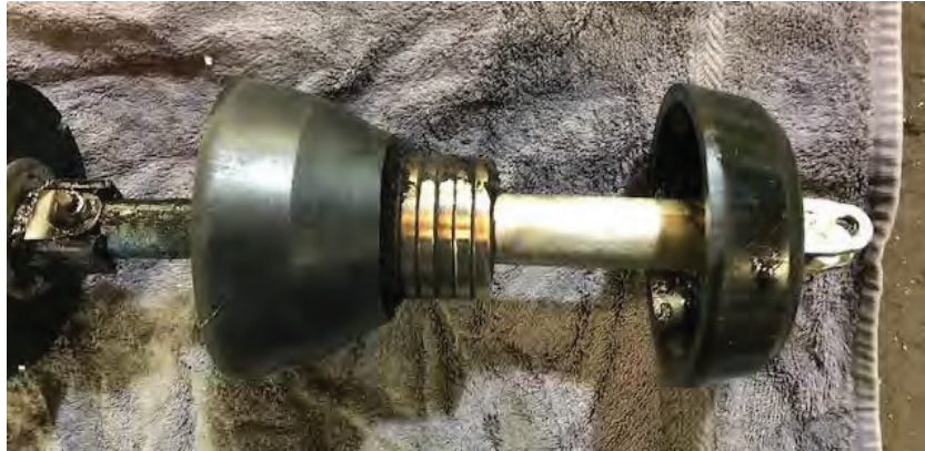
Figure 11. Drive section of the cleaning tool with magnets, post run.
