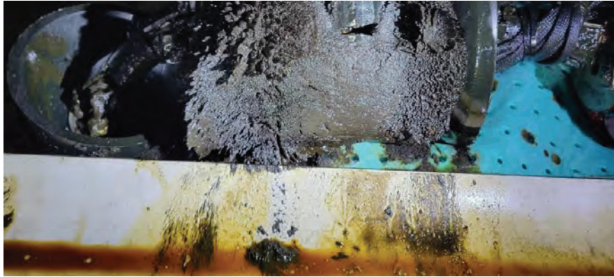
Figure 4. Ferrous debris on an MFL tool.
