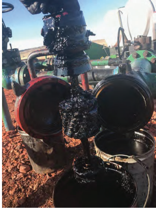
Figure 8. 4" combination gauge plate and cleaning pig, post run.
