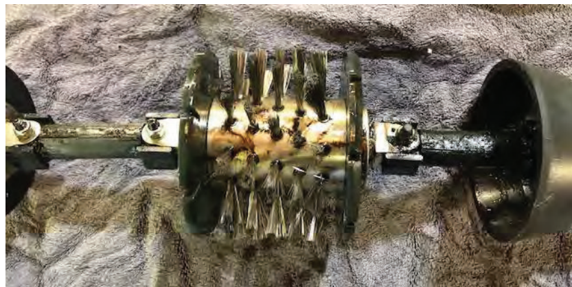
Figure 12. Brush section of the cleaning tool, post run.
