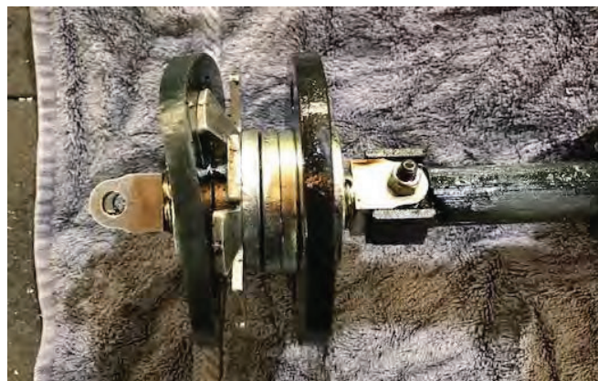
Figure 13. Gauge plate section of cleaning tool with bent tabs, post run.
