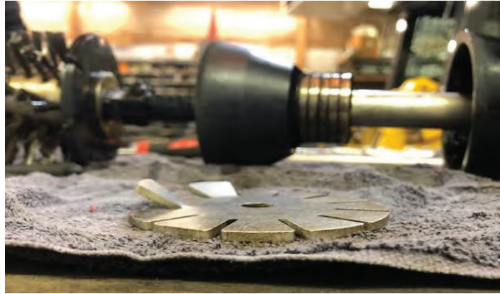
Figure 14. Cleaning tool's gauge plate showing bent tabs, post run.
