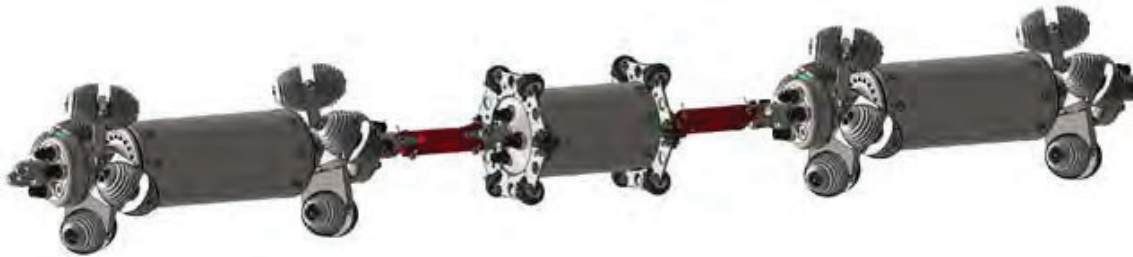
Figure 16. 10” Electro helix crawler system
