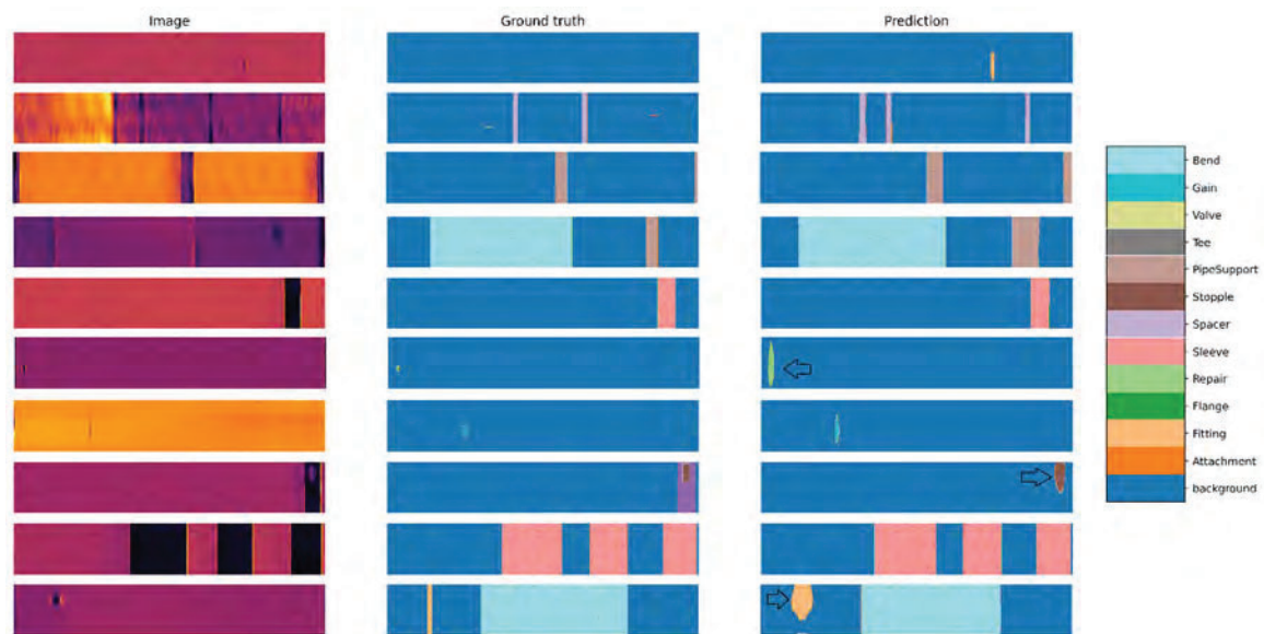
Figure 2 : Comparison of the MFL data (left) to the annotated features (middle) and predicted features (right)
