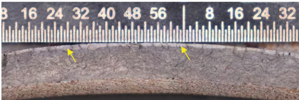
Figure 4. Fracture surface, sample DSAW2.
