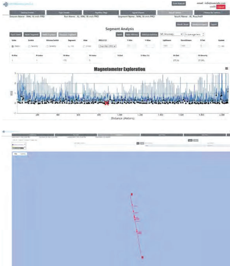
Figure 3: Screenshot from the software application used for post run analysis of MSIB magnetometer data depicting both linear reference magnetic and GIS representation. (Chevron Technical Center)
