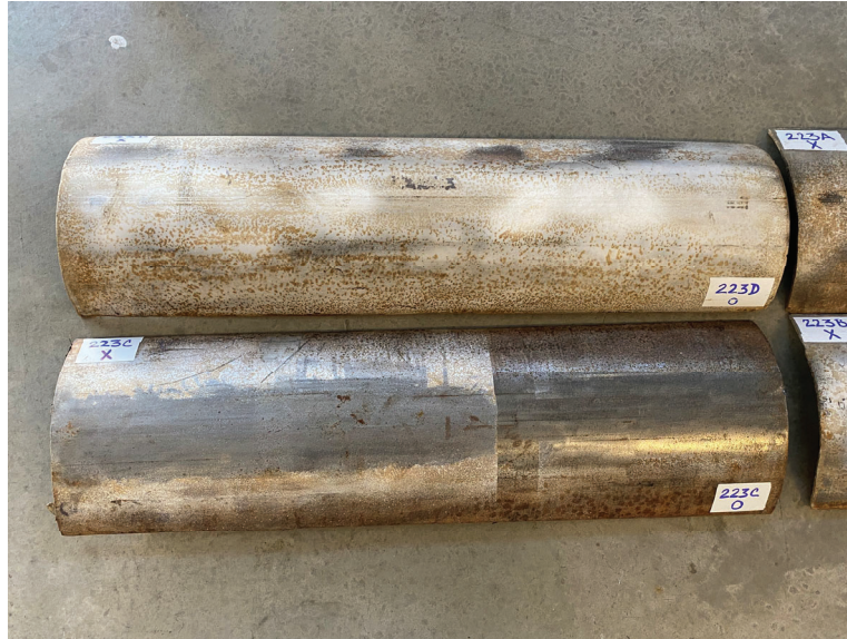
Figure 9. Example of defect sample coupons used in the ITD NDE Program
