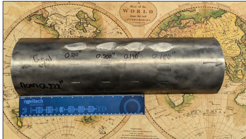
Figure 2. NPS 6 test pipe notch layout
