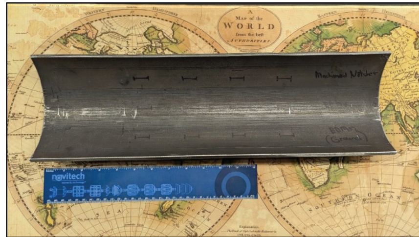
Figure 3. NPS 6 test pipe internal surface view with identified notch layout.
