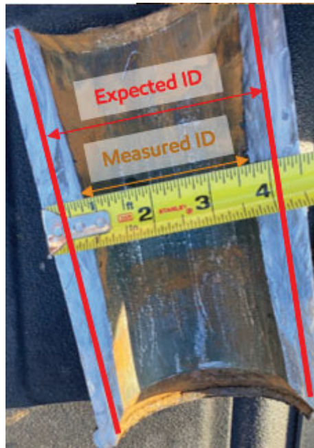
Figure 1. Cross section of typical heavy wall tee comparing expected vs actual ID.
