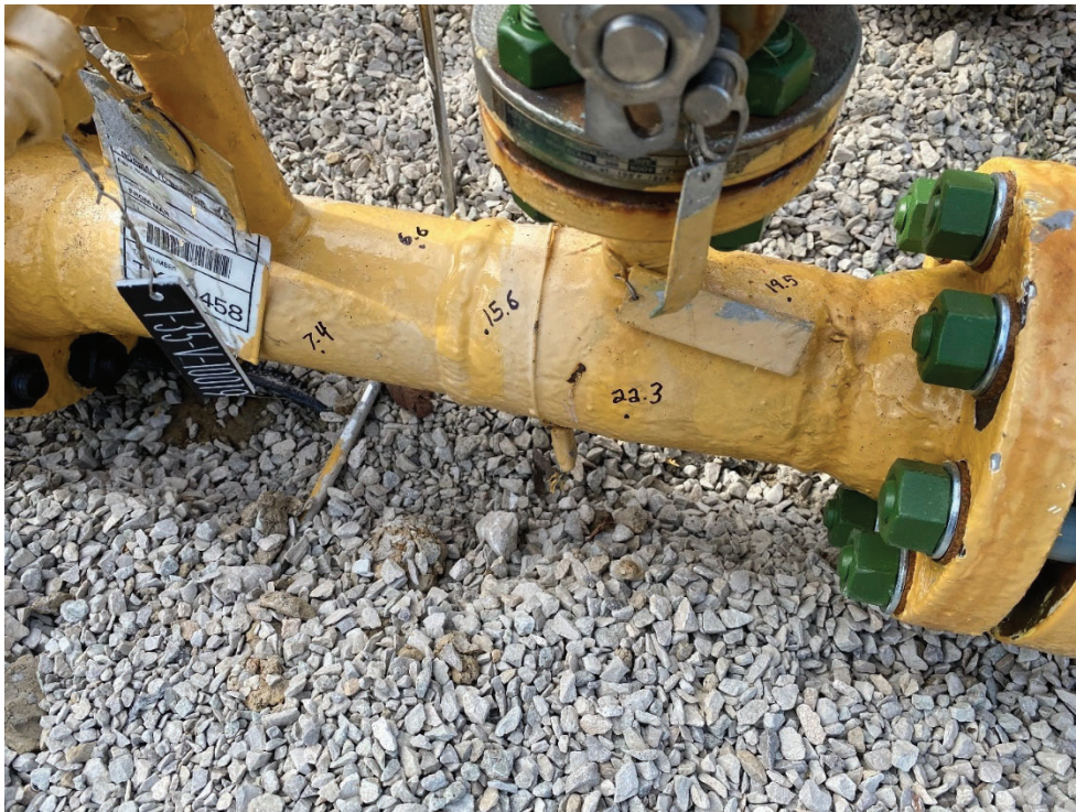
Figure 8. 3" Heavy wall tee with wall thickness up to 22.3mm (0.878"). Bore was 60.3mm (2.375"), a 20% restriction.
