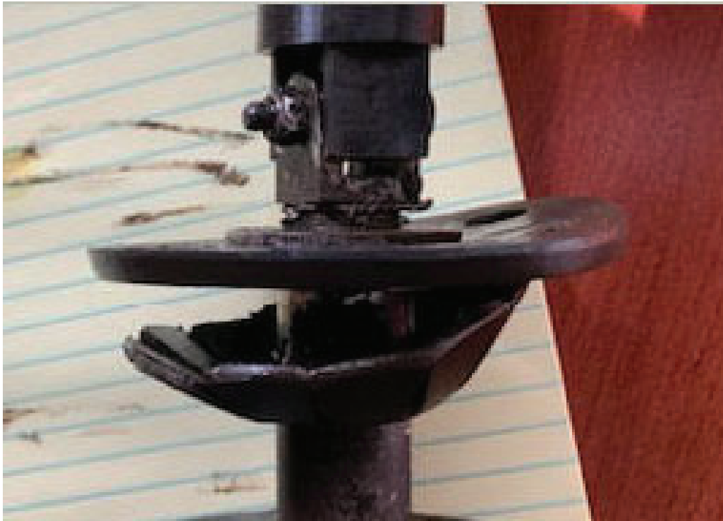
Figure 9. After construction, a KMAX gauge plate pig was run through the new pipeline.
