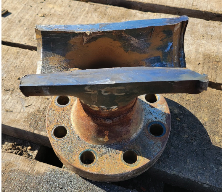
Figure 3-. Cross section of schedule 40 tee showing heavy wall thickness.
