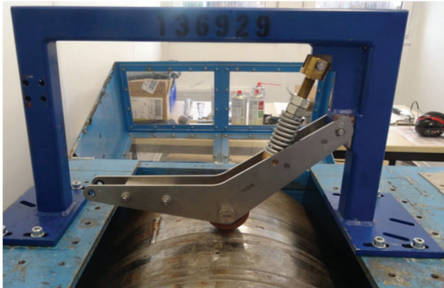
Figure 14. Endurance test system for sensor carrier wheels
