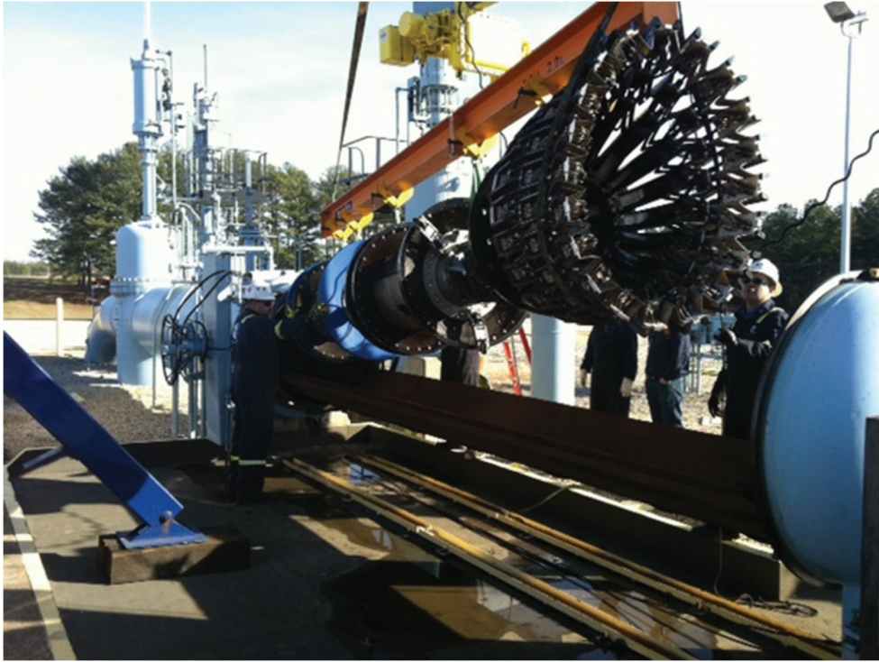
Figure 3. NDT Global UC tool in launcher with tray configuration
