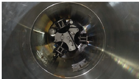
Figure 8 TRITON undergoing ACFM detection capabilities assessment.
