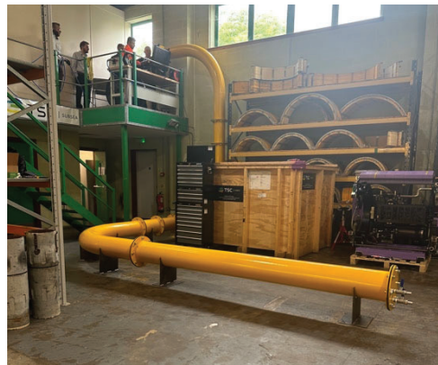
Figure 7 Full-size mock-up of the riser used to demonstrate TRITON's navigation
