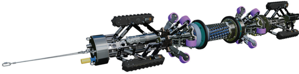
Figure 15 Dual TRITON crawler with ART Scan module
