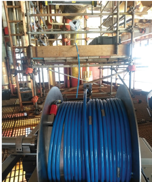
Figure 3 Umbilical management and winch system
