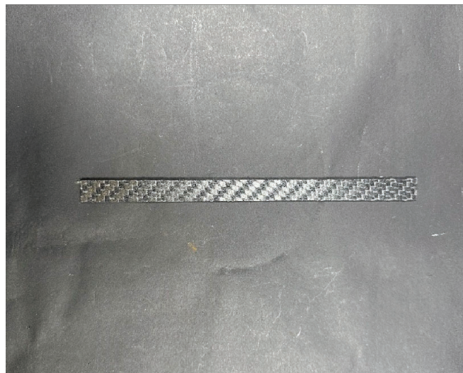
Figure 2: Prepared sample panels and specimens for tensile testing
