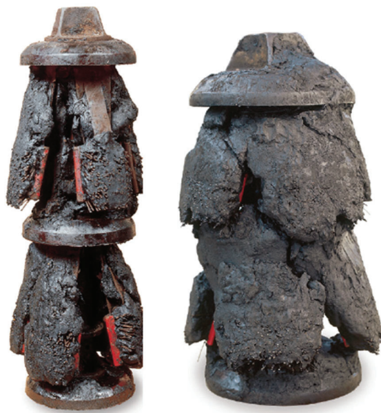
Figure 9. Lack of progressive pigging.
