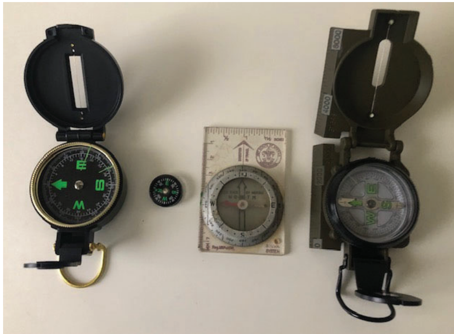
Figure 15. Compasses to assist in locating a pig or inspection tool carrying magnets.
