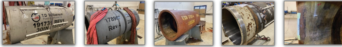
Figure 5: Photographs from the different test rigs used for gripping validation testing.
