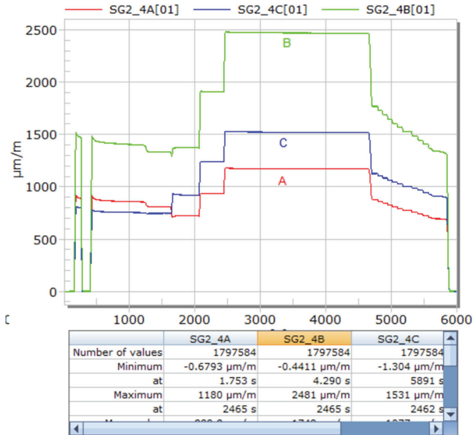
Figure 4: Graph - raw strain gauge data obtained during testing
