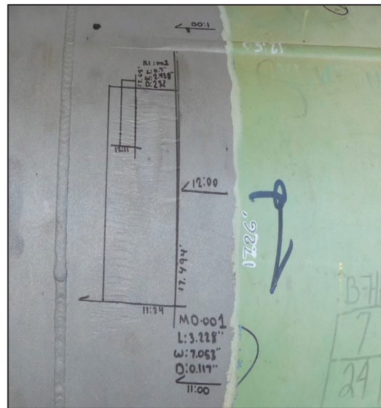
Figure 2. In situ measurement of defect area.
