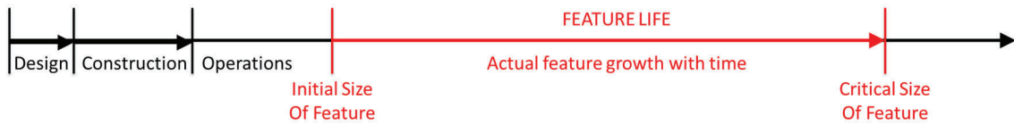
Figure 2. Timeline showing feature life from time of first initiation with feature growth until the feature's critical size is reached.
