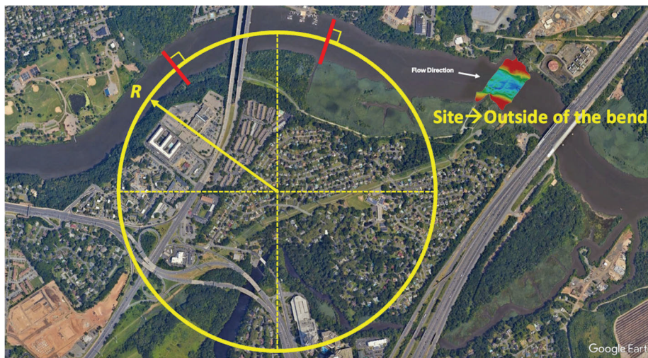
Figure 3. Example of radius of curvature ( R_c ) estimation. Red lines show the inflection points of the channel. In this case, the studied river section is located outside of the bend, so no bend scour is expected.
